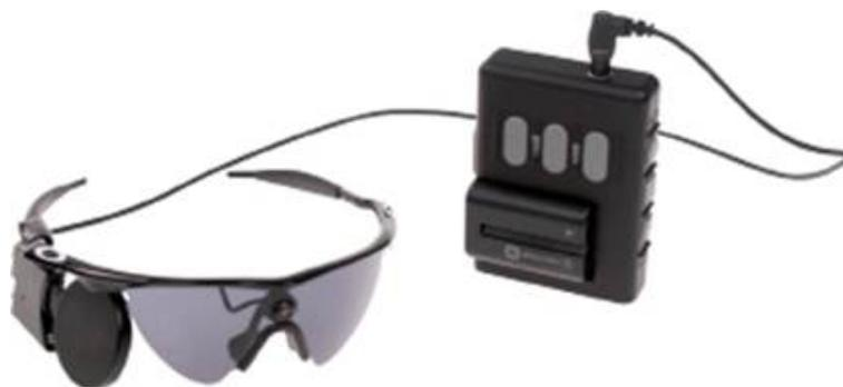
Figure 4: External Components of the Argus II System
